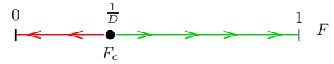
Fig. 4. Flow diagram for the fidelity F of the generalized distillation protocol for qudits given by the recursion relation (27).
